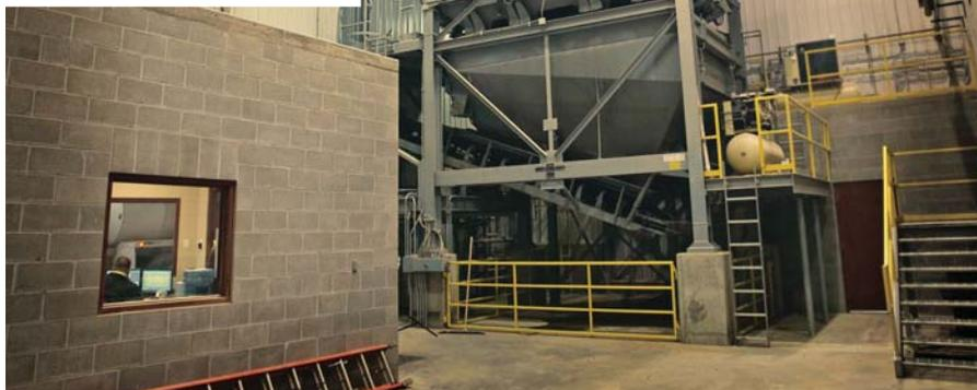
The RexCon LoGo 12 features aggregate bins and batcher enclosed by a four-story batch tower, built with Lite-Deck tilt-up wall panels and a post-tensioned concrete roof. Operations superintendent Cory Birrenkott (inset) loads a truck using the RexCon RC3 batch control system. The first load of concrete out of the Westgate Avenue plant was batched on Labor Day 2010.
